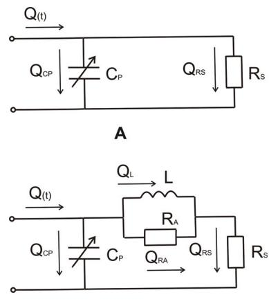
**Fig. 1.** Hemodynamical representation of two (A) and four (B) element artery models' in systole
