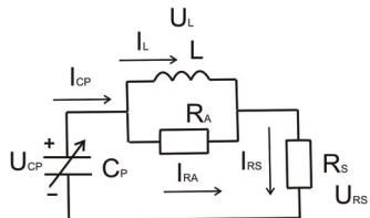
**Fig. 2.** Electrical analogy of artery model in diastole
