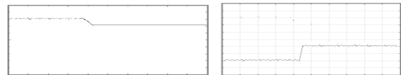
Fig. 7. Waveforms of load voltage, inductor current when switching from forward to back up mode of conduction
