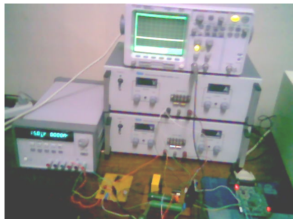
Fig. 9. Buck converter interfaced to TMS320LF2407A
