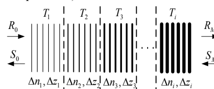
Fig.1. Transfer matrix method used to obtain the spectral characteristics of a fiber Bragg grating ( \Delta n - average index of refraction, \Delta z - section length, R_0, S_0, R_M, S_M - electromagnetic waves amplitudes)
