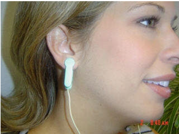
Fig. 1. Location of electrodes on the ear lobes
