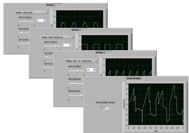
Fig. 1. The composing of the input signal
