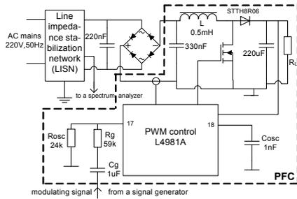
Fig. 2. Simplified schematic diagram of the experimental setup
