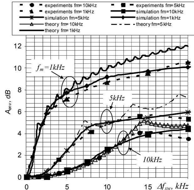
Fig. 4. Obtained attenuation  $A_{env}$  of EMI noise versus  $\Delta f_{sw}$  for different  $f_m$  resulting from the experiments, the simulations and FMT.
