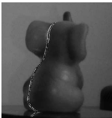
Fig. 5. Image of the elephant statue acquired by a digital video camera during laser scanning
