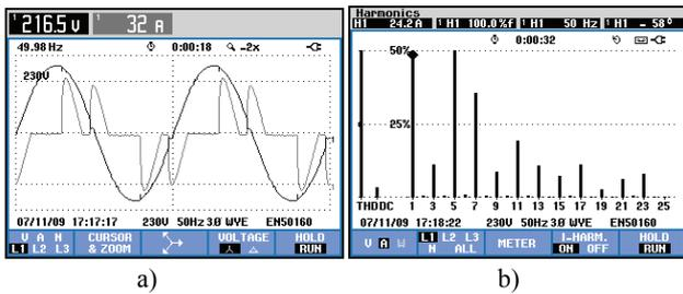
**Fig. 2.** Experimental results of the nonlinear load currents with respect to the grid voltage and the FFT spectrum of the thyristor rectifier load current obtained from Fluke 435 power quality analyzer
