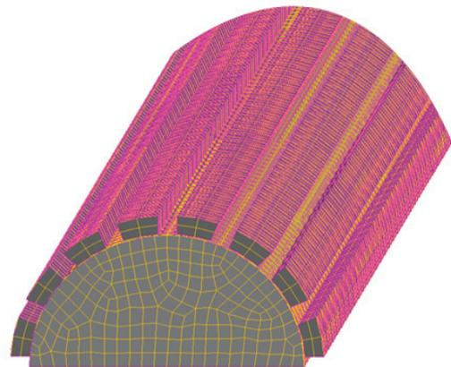
Fig. 4. Computational mesh for the water domain
