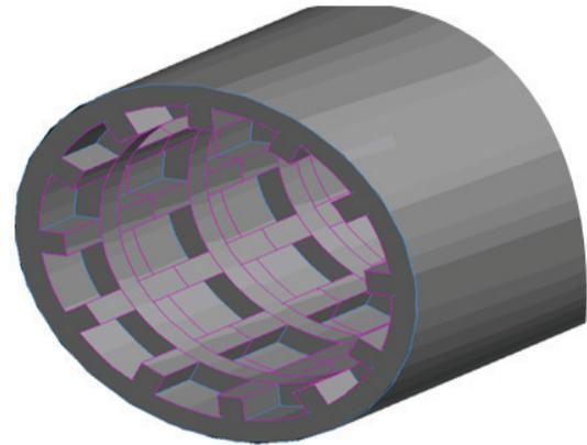
Fig. 2. 3D geometry of the heating pipe
