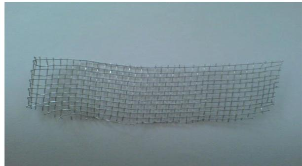
Fig. 3. Aluminium mesh
