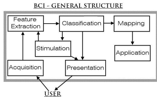
Fig. 2. General structure of a typical BCI system [8].
