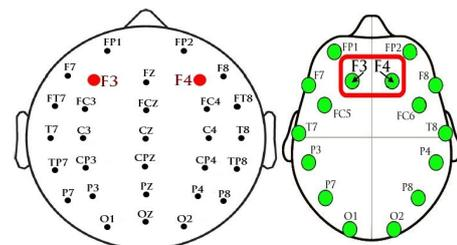
Fig. 4. Left: F3 and F4 electrodes placement, according to the 10-20 EEG electrodes placement standard; Right: F3 and F4 electrodes placement in Emotiv EPOC headset.
