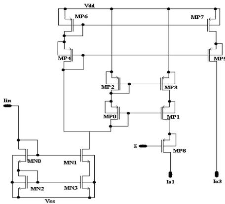
Fig. 7. Circuit schematic of a Current Division Cell
