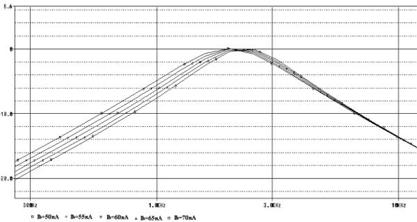
**Fig. 11.** Variation of the BPF central frequency in respect with the bias current  $I_{b3}$
