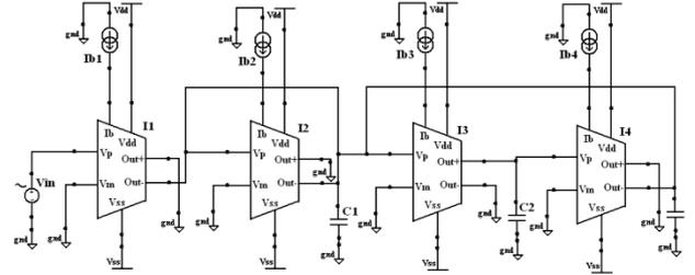
**Fig. 4.** Circuit schematic of the Gm-C biquad
