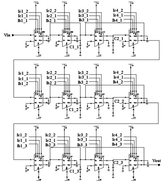
**Fig. 5.** The 6<sup>th</sup> order Butterworth approximation BPF schematic
