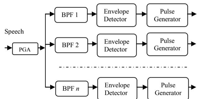
Fig. 2. Block diagram of the CIS processing
