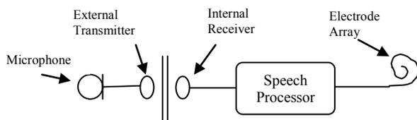
Fig. 1. Implantable system of a transcutaneous CI
