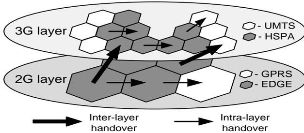
Fig. 1. Overlapping mobile data access networks
