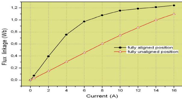
Fig. 7. Flux linkage profile of the actuator
