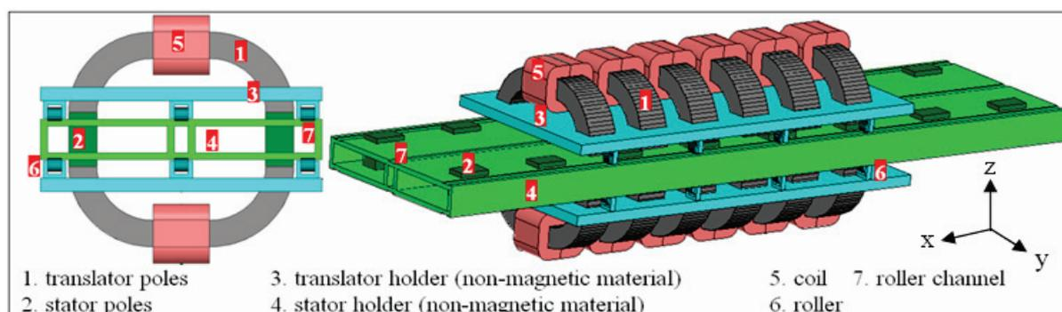
Fig. 1. Simulated model of the linear actuator
