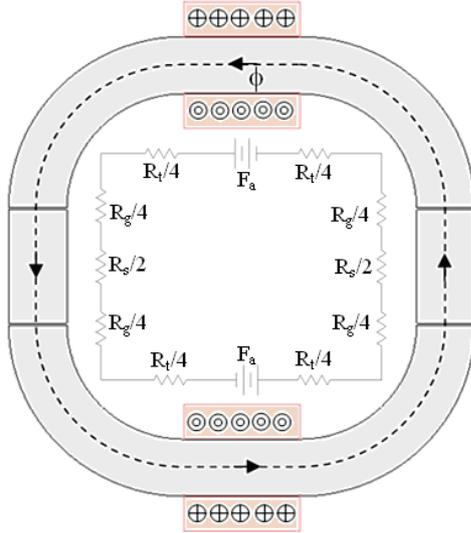
Fig. 5. Actuator core flux path and magnetic circuit
