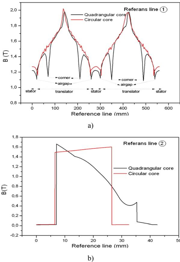
**Fig. 10.** Magnetic flux density in the reference lines: a – 1st reference line; b – 2nd reference line
