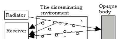
Fig. 1. LIDARs working principle
