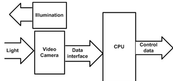
Fig. 2. Typical structure of image processing system
