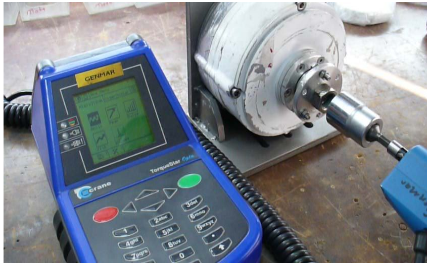
Fig. 2. The setup of the cogging torque measurement system of the designed and manufactured PMSG.
