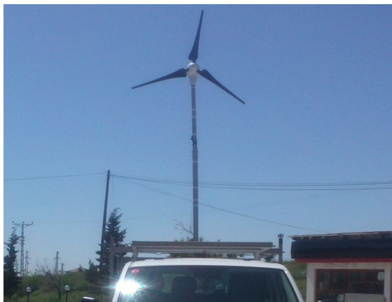
Fig. 3. Trucker testing for MWT having PMSG without and with the pole shifting.
