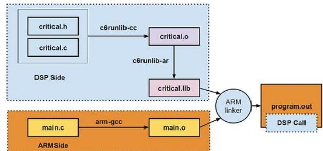
Fig. 4. C6RunLib build mechanism.
