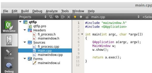
Fig. 3. Project tree of the pre-processor application.
