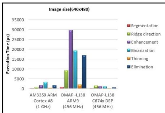
Fig. 5. Execution time on different cores using  $640 \times 480$  sized image.
