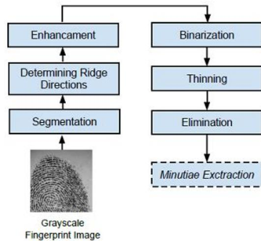
Fig. 1. The pre-processing algorithms used in minutiae based fingerprint analysis.
