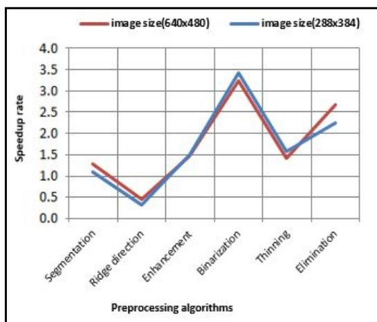
Fig. 6. The speedup ratio of pre-processing algorithms.
