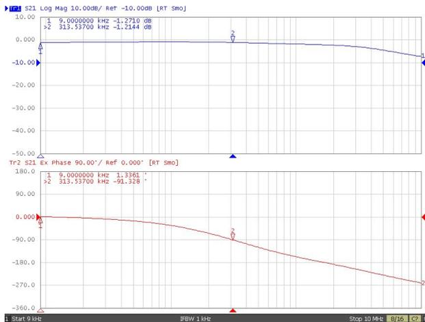
Fig. 8. All-pass filter response for  $g_m = 1$  mS,  $R_x = 2$  k $\Omega$  and  $B = 1$ .
