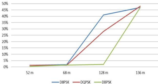
Fig. 6. Variation of BER value for PLC communication in selected LV network structure under 10 % full band noise and with FEC applied.
