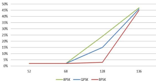
Fig. 9. Variation of BER value for PLC communication in selected LV network structure under influence of 1kV impulse disturbance without FEC applied.
