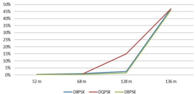
Fig. 7. Variation of BER value for PLC communication in selected LV network structure under 10 % full band noise and without FEC.
