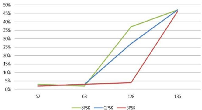
Fig. 8. Variation of BER value for PLC communication in selected LV network structure under influence of 1 kV impulse disturbance with FEC applied.
