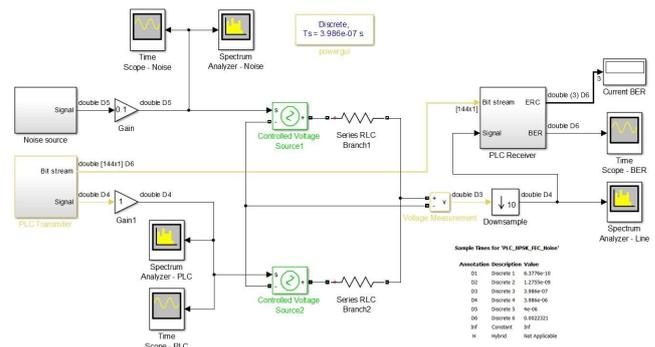
Fig. 1. General idea of simulation PRIME PLC over power system network.
