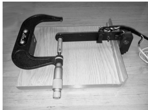
Fig. 5. Micrometer screw for bending the steel beam with mounted: heater, temperature sensor (Pt100) and two strain gauges.
