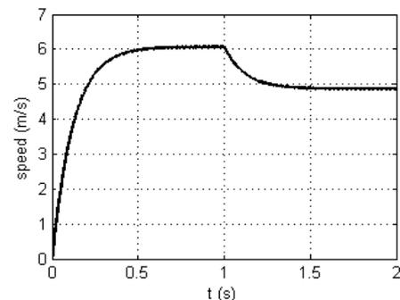
Fig. 5. Uncontrolled ELS speed response.
