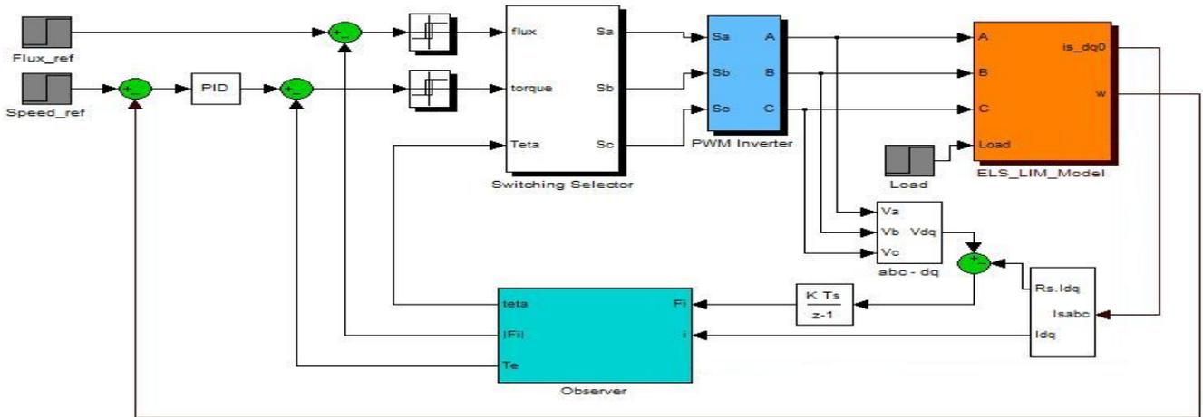
Fig. 2. DTC scheme of Linear Electromagnetic Launcher system.
