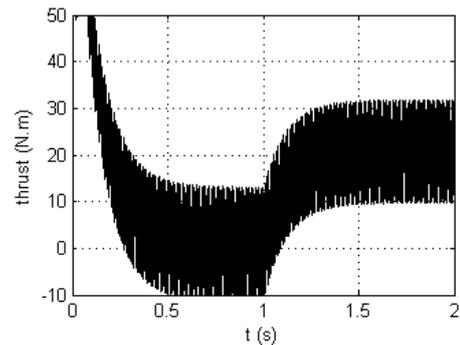
Fig. 3. Uncontrolled ELS thrust response.
