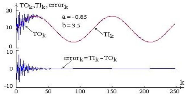
Fig. 6. The tracking error of the sinusoidal signal is very small.
