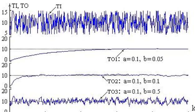
Fig. 8. For the lower “b” noise rejection is better, but PLL is slower.
