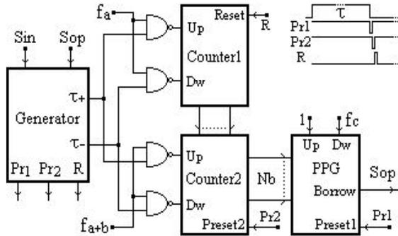
Fig. 3. The functional scheme of PLL of the second order.
