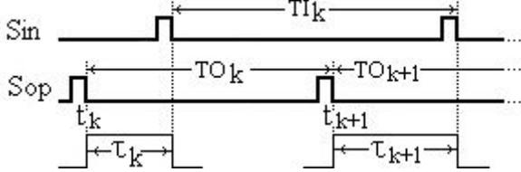
Fig. 1. The input and output variables of PLL:  $TI_k$ ,  $TO_k$  and  $\tau_k$ .
