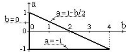
Fig. 2. The region of parameters “a” and “b” for the stable PLL.
