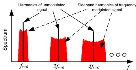
Fig. 2. Simulated spectra of unmodulated and frequency modulated input current.
