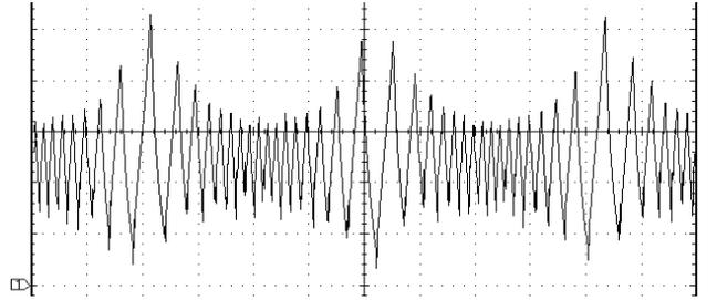
Fig. 4. FM buck converter power inductor current without core saturation effects. Parameters:  $f_{sw}=100\text{kHz}$ ;  $f_m=5\text{kHz}$ ;  $\Delta f_{sw}=35\text{kHz}$ . (Scale: 50us/div; 100mA/div).
