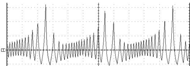
Fig. 6. FM buck converter output capacitor current when core enters saturation. Parameters:  $f_{sw0}=100\text{kHz}$ ;  $f_m=5\text{kHz}$ ;  $\Delta f_{sw}=35\text{kHz}$ . (Scale: 50 $\mu\text{s}/\text{div}$ ; 400mA/ $\text{div}$ ).
