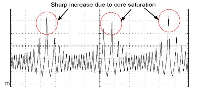
Fig. 5. FM buck converter power inductor current with core saturation effects. Parameters:  $f_{sw}=100\text{kHz}$ ;  $f_m=5\text{kHz}$ ;  $\Delta f_{sw}=35\text{kHz}$ . (Scale: 50us/div; 400mA/div).
