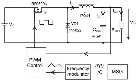
Fig. 1. Schematic of FM closed-loop buck converter used.
