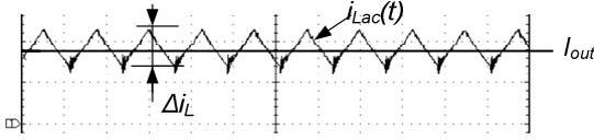
Fig. 3. Unmodulated buck converter power inductor current. (Scale: 10us/div; 100mA/div).
