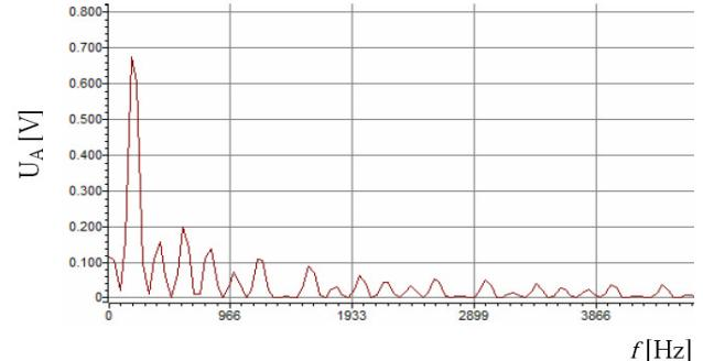
Fig. 13. Amplitude spectrum of square waveform.
