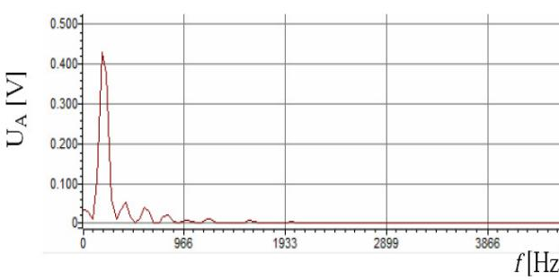
Fig. 11. Amplitude spectrum of triangular waveform.
