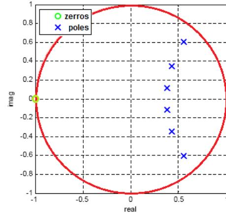
Fig. 5. Distribution of poles and zeros of proposed filter.
