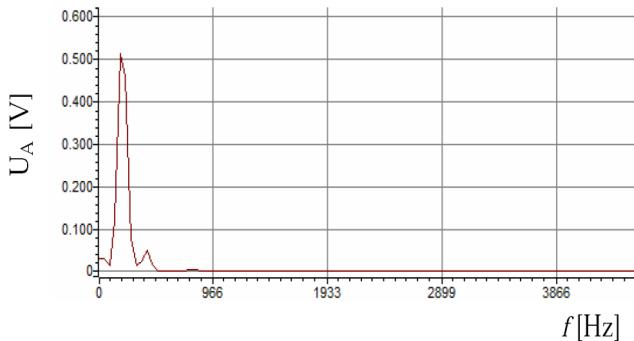
Fig. 9. Amplitude spectrum of sinusoidal waveform.
