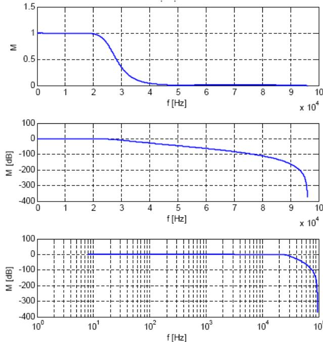
Fig. 4. Frequency characteristic of proposed filter.
