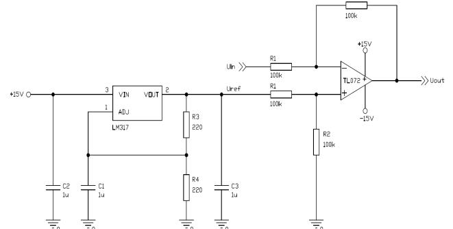
Fig. 3. Block scheme of circuit for voltage adjustment.
