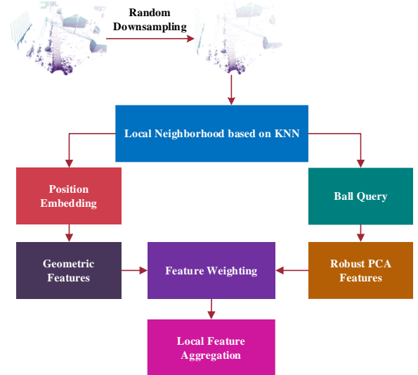
Fig. 3. Point branch of the sparse convolution.
