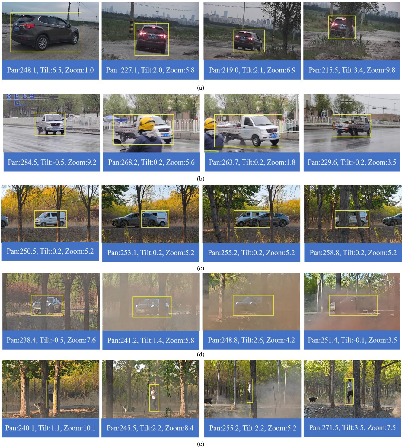
Fig. 12. Qualitative results of the proposed SCAAT tracker in real-world field tests: (a) Tracking the vehicle on a sunny day; (b) Tracking the vehicle under rain and occlusion; (c) Tracking the vehicle under occlusion; (d) Tracking the vehicle under smog and occlusion; (e) Tracking the person under smog and occlusion.
