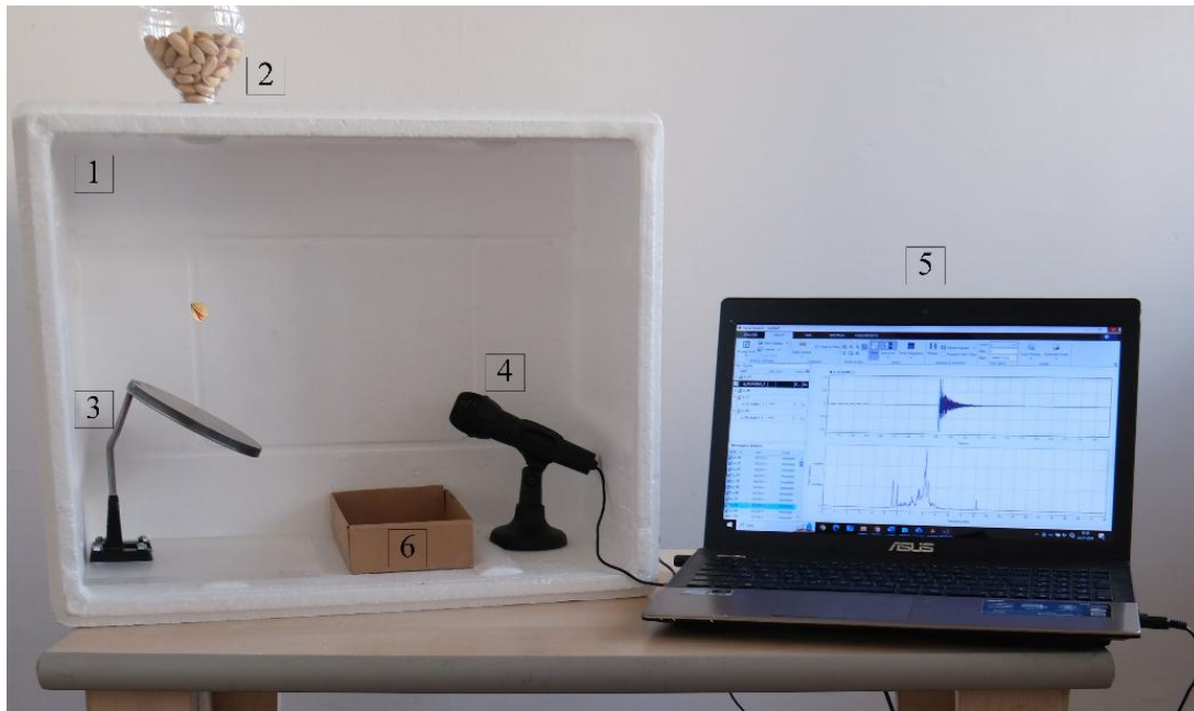
Fig. 6. Schematic of the pistachio classifier based on acoustic emissions.
