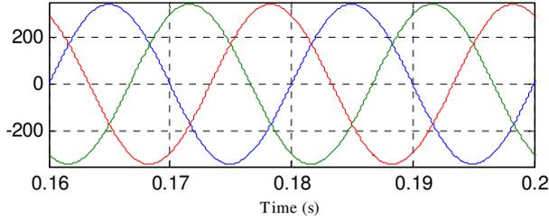
Fig. 3. Three phase balanced and undistorted (ideal) grid voltages.
