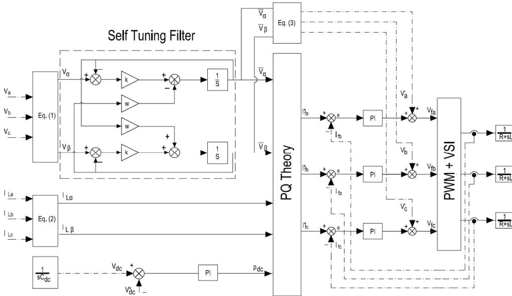
Fig. 2. The block scheme of the proposed control system.
