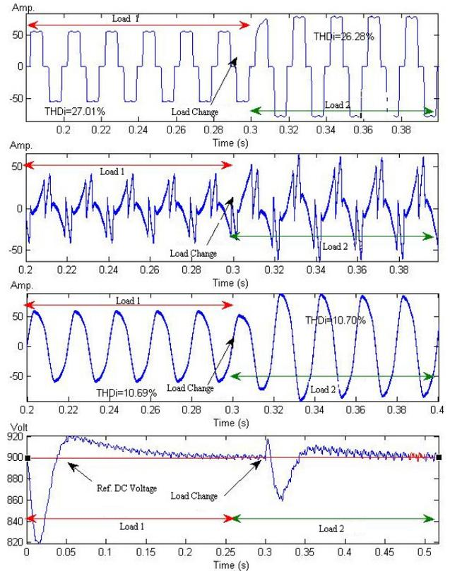
Fig. 6. Performance of the APF under non-ideal grid voltage and step-up load change. Top waveform: Load current of phase a. Compensating current of phase a. Grid current of phase a. Bottom waveform: DC link capacitor voltage.
