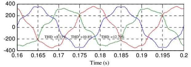
Fig. 5. Three phase unbalanced and distorted (non-ideal) grid voltages.
