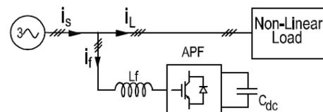
Fig. 1. Block diagram of the APF.
