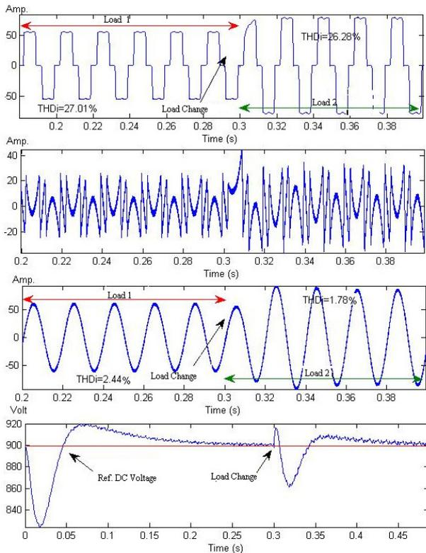
Fig. 7. Performance of the STF based APF under non-ideal grid voltage and step-up load change. Top waveform: Load current of phase a. Compensating current of phase a. Grid current of phase a. Bottom waveform: DC link capacitor voltage.
