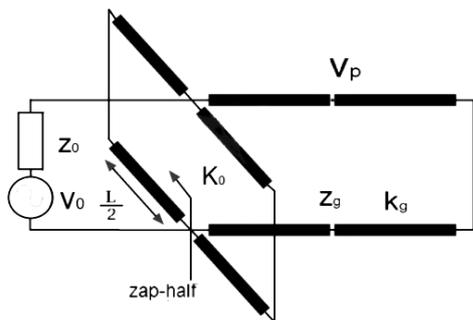
Fig. 2. Impedance of aperture and its equivalent circuit.
