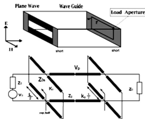
Fig. 5. The equivalent circuit for an enclosure with aperture load.
