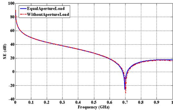
Fig. 6. Different SE for an aperture load enclosure and a short circuit enclosure based on TL model.
