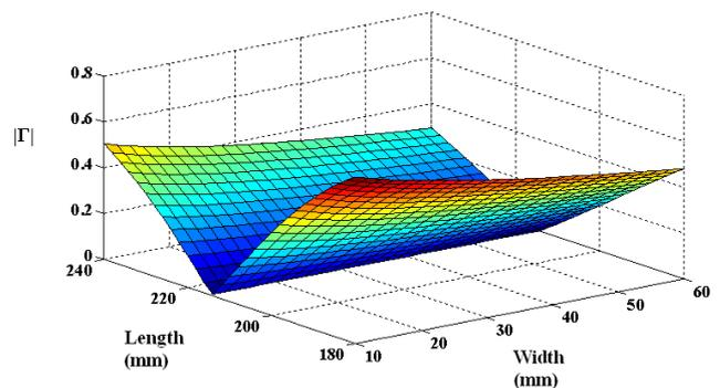
Fig. 9. Reflection coefficient for different length and width at f=0.7 GHz
