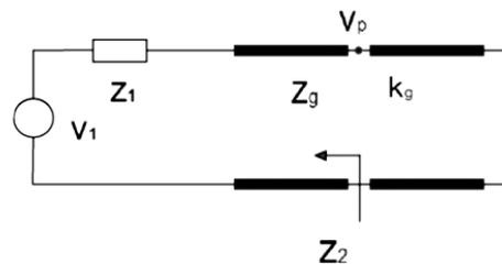
Fig. 3. Thevenin equivalent circuit.
