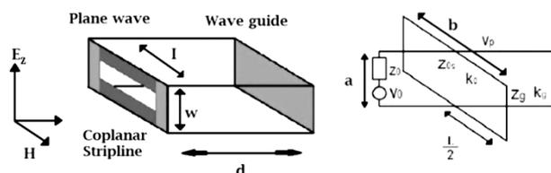
Fig. 1. Rectangular enclosure with an aperture and its equivalent circuit (a=300 mm, b=120 mm, d= 300 mm), (l=100 mm, w=15 mm).
