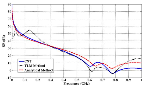
Fig. 11. Evaluation of shielding effectiveness parameter by using different methods.
