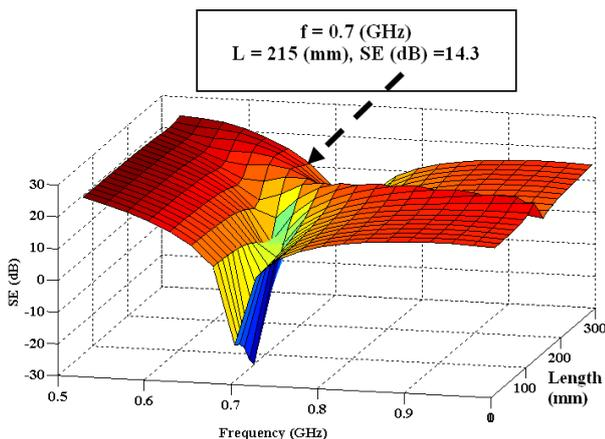
Fig. 7. Shielding effectiveness versus frequency and length.
