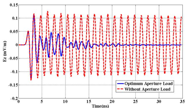
Fig. 10. Time domain electric field strength at the centre of aperture.
