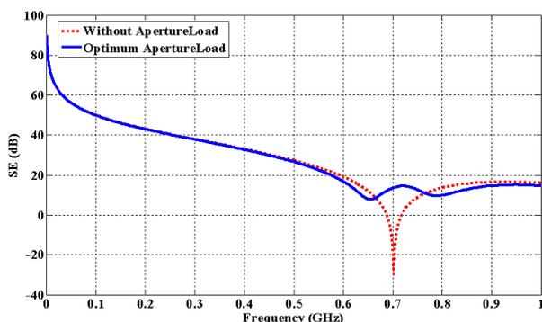
Fig. 8. Comparison of SE parameter of optimum aperture load and short circuit shielding box by using TL model.
