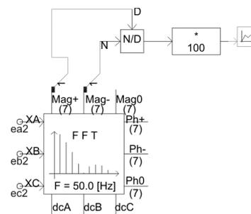
Fig. 5. Unbalance measuring scheme in PSCAD.
