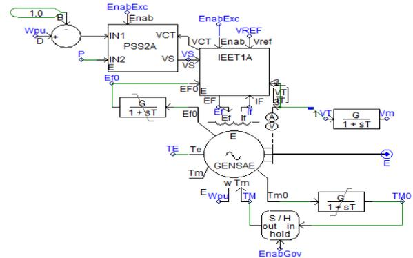
Fig. 4. PSCAD model of CHP generator.
