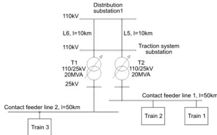
Fig. 2. Electric railway traction system connection scheme.
