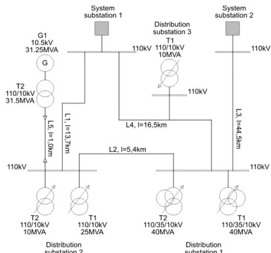
Fig. 1. Principal scheme of electrical transmission network.
