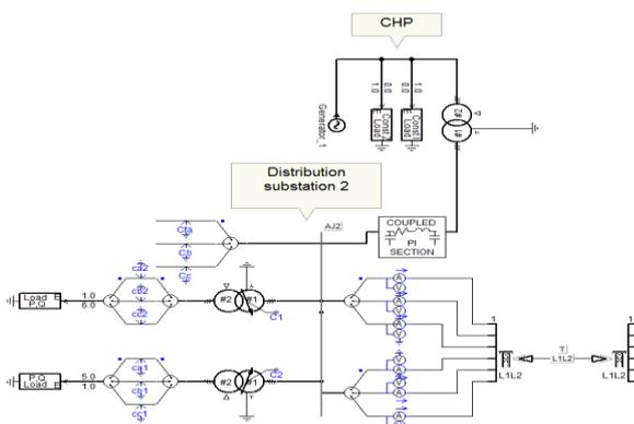
Fig. 3. PSCAD model fragment of distribution substation 2 and CHP plant.
