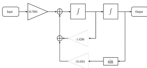
Fig. 3. Simulink pendulum model. The gains were adjusted based on the physical pendulum structure.
