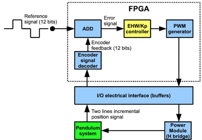
Fig. 10. Simplified FPGA content diagram.
