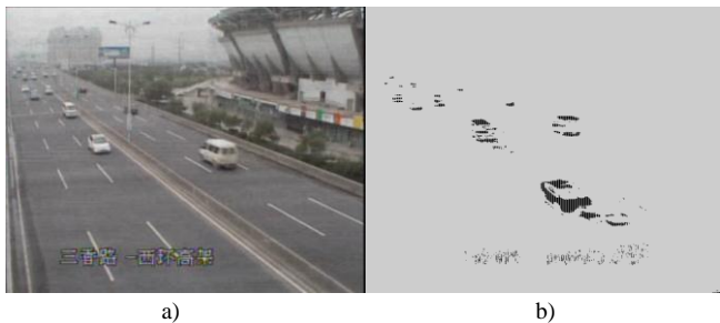
Fig. 4. The left figure is snapshot monitoring system in highway. The right figure is the greyed image after separating moving objects and removing its shadow.
