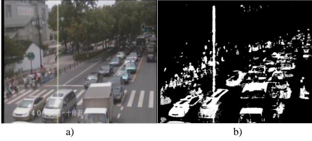
Fig. 5. The image with reflection light band.
