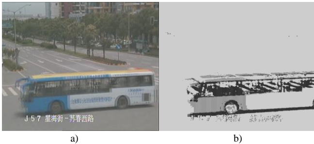
Fig. 3. The left figure is snapshot from monitoring system in urban road. The right figure is the greyed image after separating moving objects and removing its shadow.
