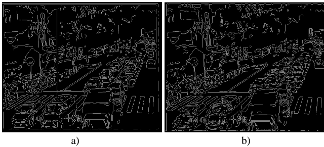
Fig. 7. The left figure is the edge detected by Canny algorithm before reflection light band erasing; the right figure is the edge detected by Canny algorithm after reflection light band erasing.
