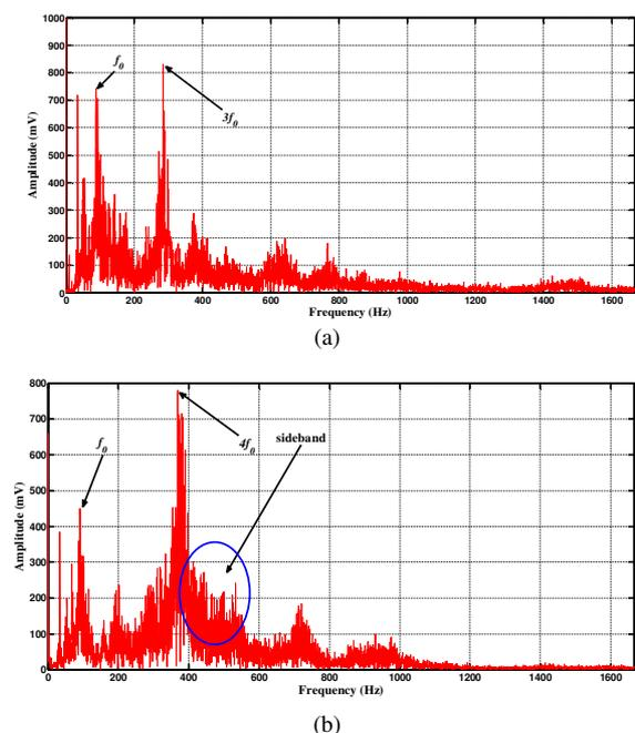
Fig. 2. The engine vibration signals: (a) the original vibration signal and (b) the fused vibration signal using ICA.
