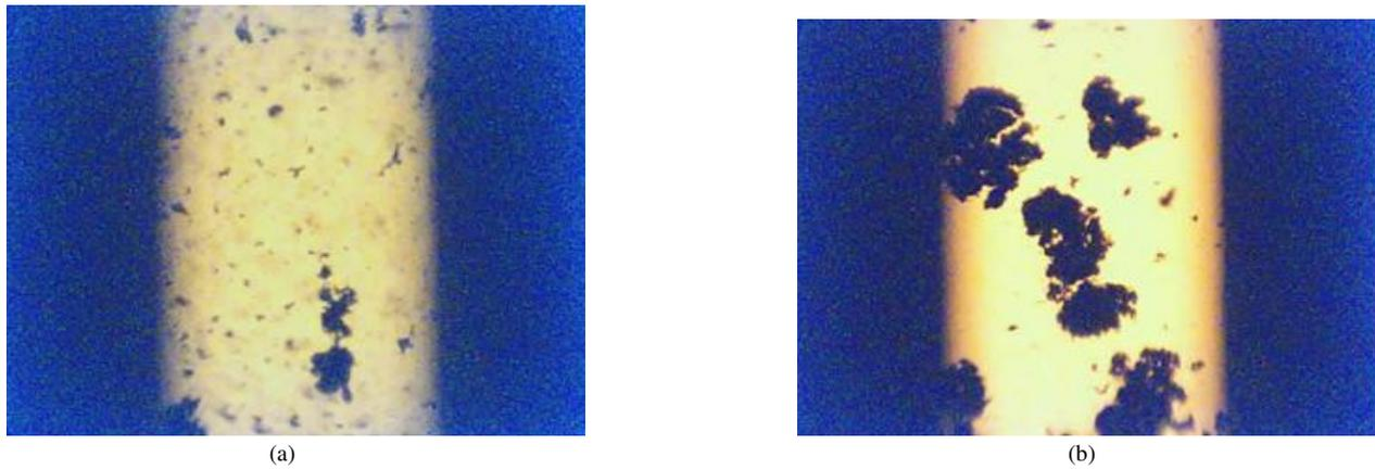
Fig. 3. The engine wear particles: (a) particles in normal condition and (b) particles in faulty condition.
