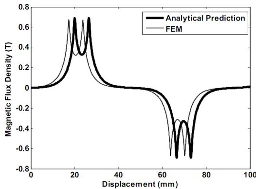
Fig. 3. X component of the flux density in the middle of the air gap.
