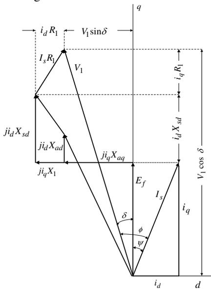
Fig. 10. The vector diagram of the synchronous motor.
