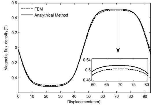
Fig. 5. Y component of the flux density in the middle of the magnetic air gap.
