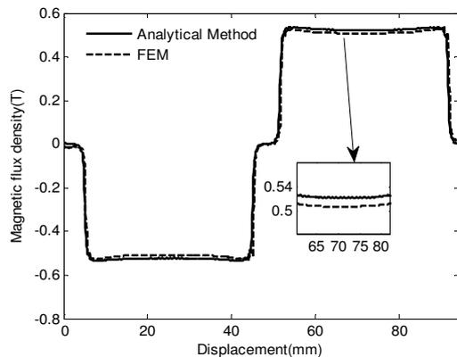
Fig. 4. Y component of the flux density in the middle of the air gap.
