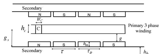
Fig. 1. The structure of ACPMLSM.
