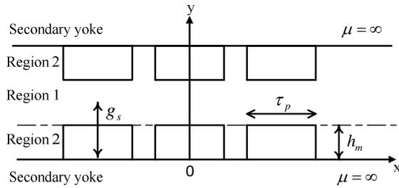
Fig. 2. Analysis model of an ACPMLSM.
