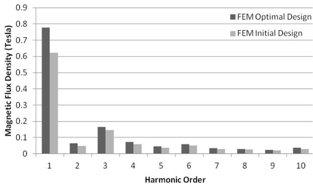
Fig. 12. Harmonic contents of y component flux density produced by the PMs before and after optimization.
