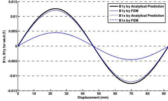
Fig. 9. The vertical and the horizontal components of the air gap flux density generated by the primary currents at  $\omega t=0$  using analytical method and FEM.
