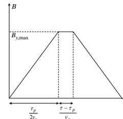
Fig. 11. Flux density variations in the yoke [14].
