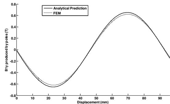
Fig. 7. The first harmonic of vertical component of the air gap flux density produced by the PM using analytical method and FEM.
