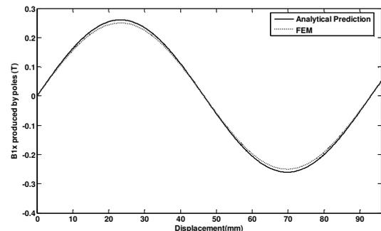
Fig. 8. The first harmonic of horizontal component of the air gap flux density produced by the PM using analytical method and FEM.
