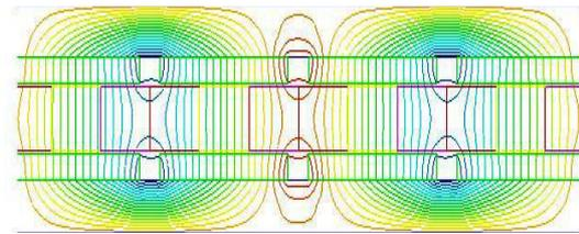
Fig. 6. Flux lines at the center of the motor.
