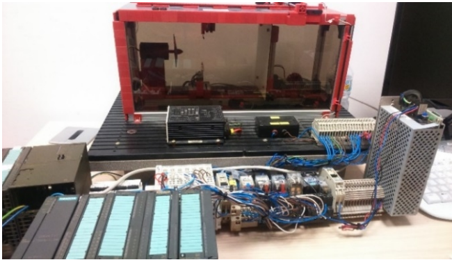
Fig. 6. Climate room model where the sensors and actuators are connected to the PLC device.
