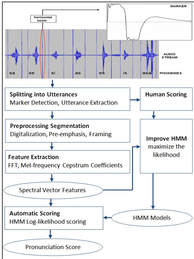
**Fig. 1.** The architecture of automatic pronunciation scoring system
