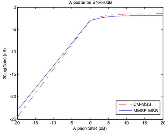
**Fig. 1.** Gain function of the proposed estimator and MMSE-MSS estimator
