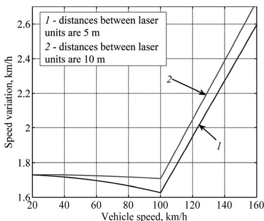
Fig. 4. Maximum vehicle speed variation (to achieve  $\pm 1$  km/h expanded uncertainty (speed is below 100 km/h) and  $\pm 1\%$  (speed is above 100 km/h))
