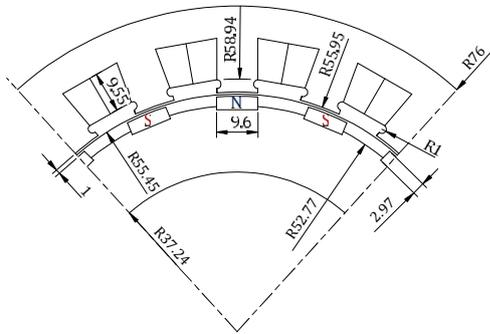
Fig. 3. Base dimensions of PMSG in cross section ( $Z_1 = 18$ ,  $2p = 16$ ). Except the slot opening and PM's pole pair number  $p$  and width  $w_{PM}$ , which are variable. Sizes in mm.
