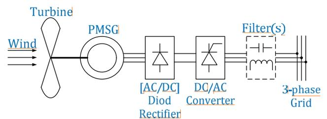
Fig. 1. PMSG in the circuit of WPP.
