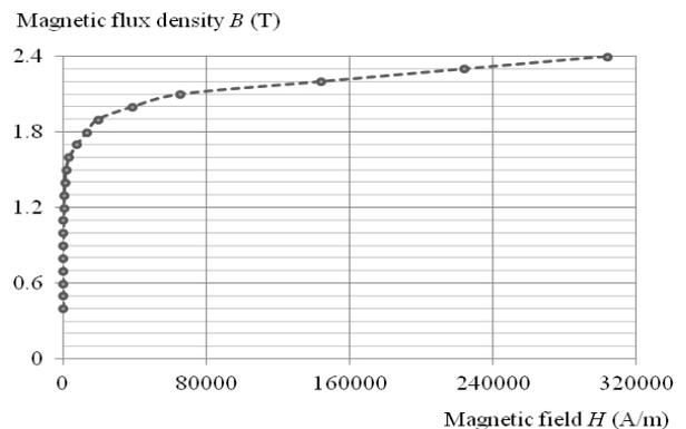
Fig. A-1. Magnetization curve for steel grade M530-50A5.
