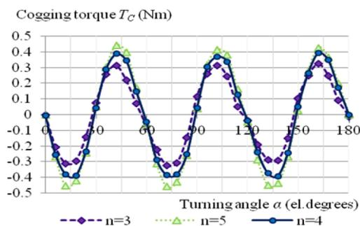
Fig. 9. Curves of cogging torque for different coefficients  $\beta$  ( $n = 4$ ).
