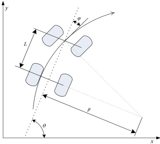
Fig. 1. A four wheeled robot configuration representation
