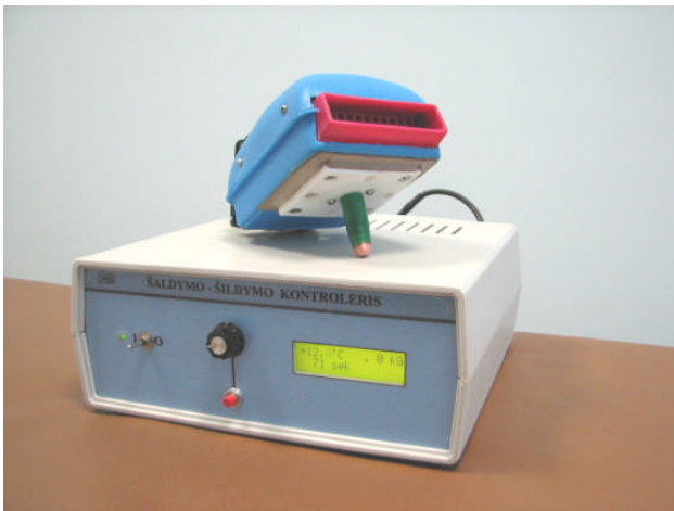
Fig. 1. View of the cold – heat contrast and local compression therapy device
