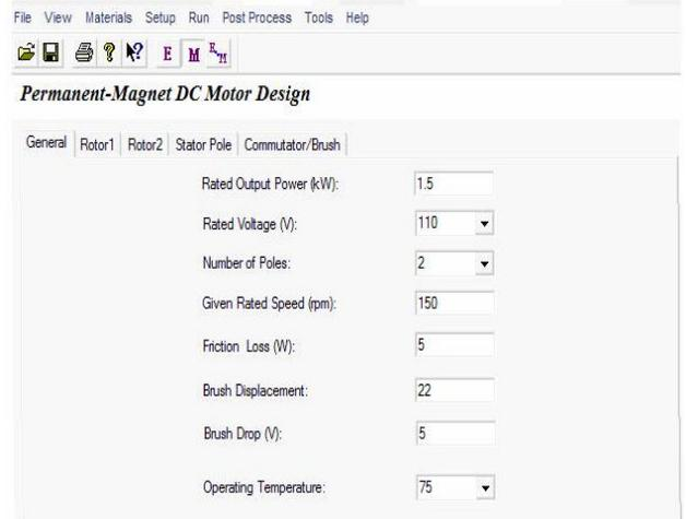
Fig. 3. Analytic design program window of brushed DC motor with 1.5 kW, 110 V, 150 rpm permanent magnet
