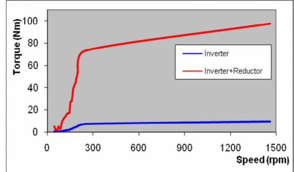
**Fig. 2.** Torque-speed curves obtained from operating the motor by feeding AC motor with inverter and by combining reductor to its shaft
