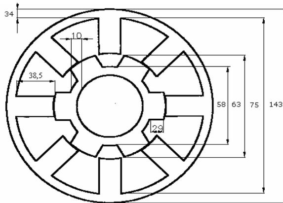
Fig. 8. Iron sheet package view and measurements (mm) of a 1.5 kW, 380 V, 150 rpm, 8/6 pole SR motor.
