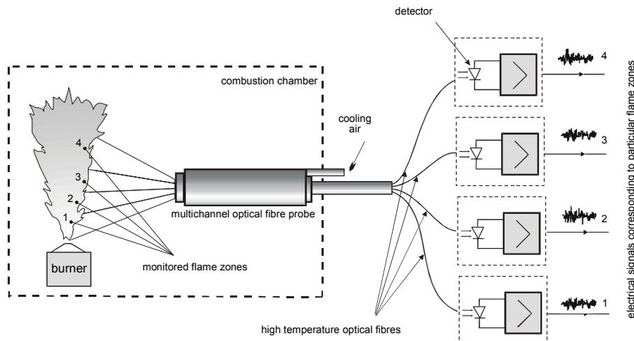
Fig. 2. Block diagram of flame monitoring system
