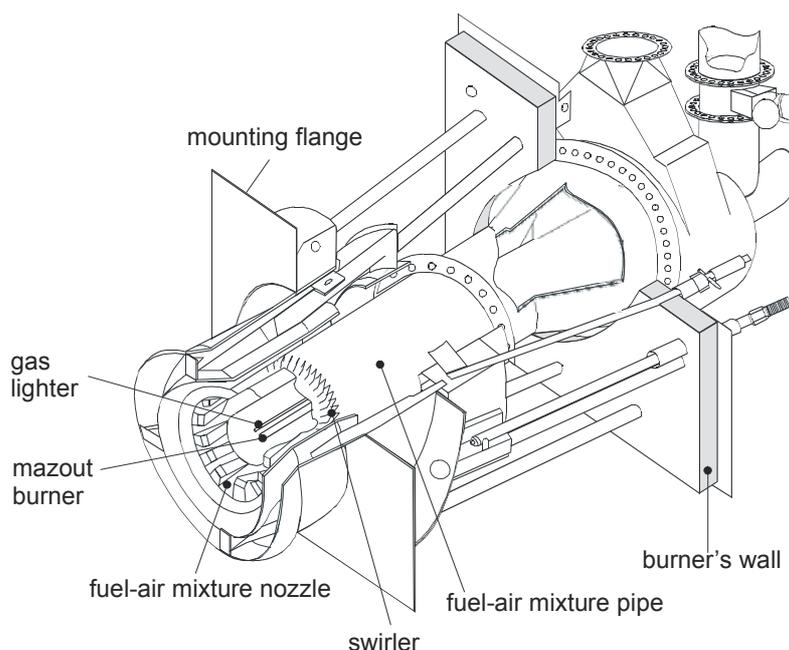
Fig. 1. Pulverised-coal burner with location of mazout burner
