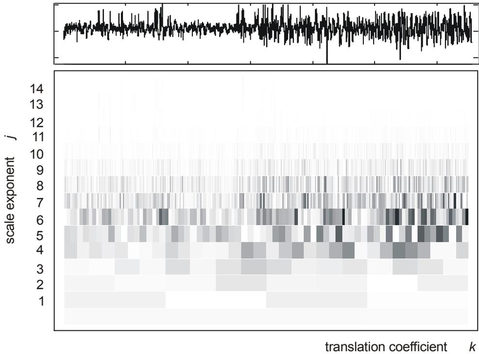
**Fig. 6.** Scalogram of discrete wavelet transform together with signal being analysed
