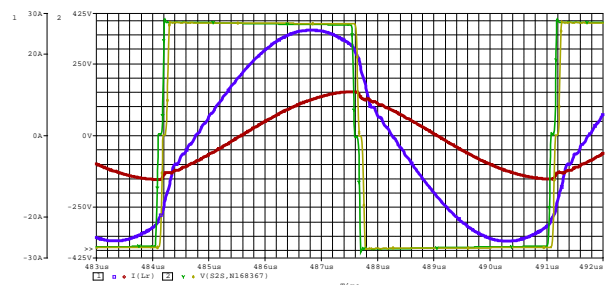
Fig. 13. Simulated waveforms of u_p(t) ( FULL LOAD, LIGHT LOAD ), and i_p(t) ( FULL LOAD, LIGHT LOAD ), at U_{in}=780 \text{ V} , f_s =143,6 \text{ kHz}
