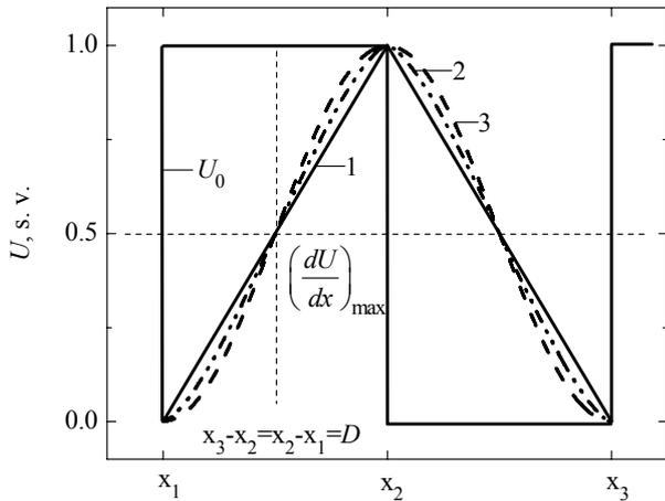
**Fig. 2.** Accepted character of surface potential  $U_0$ , which characterizes informative area and measured the potential, when electrode's tip and informative area are such: quadrate-strip (1), circle-strip (2), circle-circle (3).
