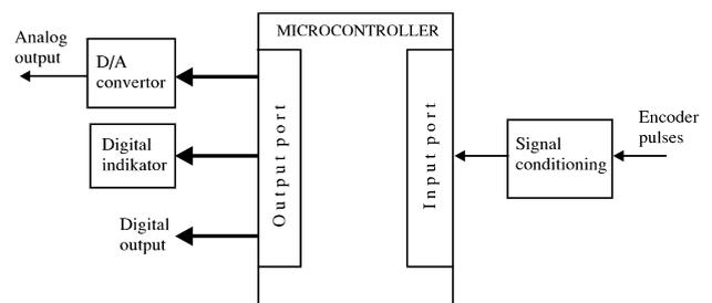
**Fig. 7.** Block diagram of the realized digital tachometer
