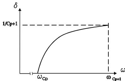
Fig. 2. Relative error versus the rotation number on the segment between two measurable rotation numbers
