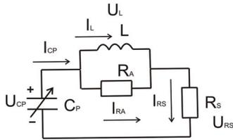
Fig. 2. Electrical analogy of artery model in diastole
