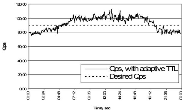
Fig. 5. DNS query rate after adaptive TTL adjustment
