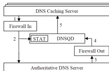
Fig. 4. Adaptive TTL adjustment program DNSQD scheme
