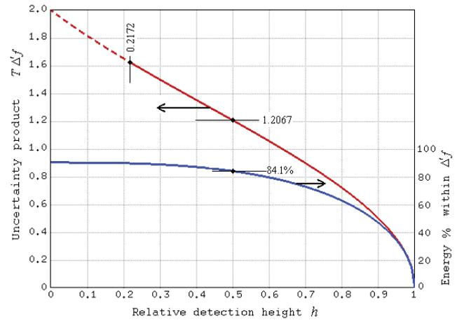
**Fig. 4.** The time-frequency uncertainty (duration-bandwidth spreading) product  $T \Delta f$  dependence on the selection of the relative height parameter  $h$  for spectral peak width detection in the case of the rectangular pulse (see Fig. 3). The corresponding energy content of the frequency interval  $\Delta f$  near the main spectral peak is displayed by the right y-axis
