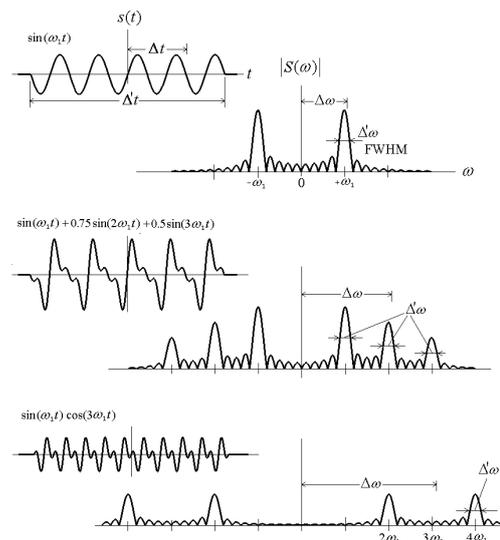
**Fig. 1.** The problematic tasks of pulse train signal (left) to Fourier spectrum (right) transforms for what the conventional methodology yields artificially increased uncertainty product values. The standard deviations  $\Delta t, \Delta \omega$  are shown in comparison with one possible alternative definition: full pulse train duration in time domain  $\Delta' t$  and the full width at half maximum (FWHM) of main spectral peaks  $\Delta' \omega$
